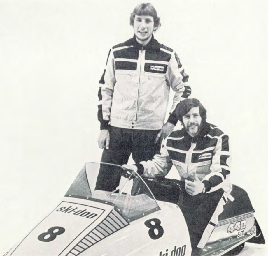
Ski-Doo Racing Team Drivers Bobby Donahue (left) and Doug Hayes are shown with one of the Super Mod Ski-Doo snowmobiles they're riding on the SnoPro circuit this season. The sled features all-new body design, independent front suspension, increased horsepower, and low center of gravity.
