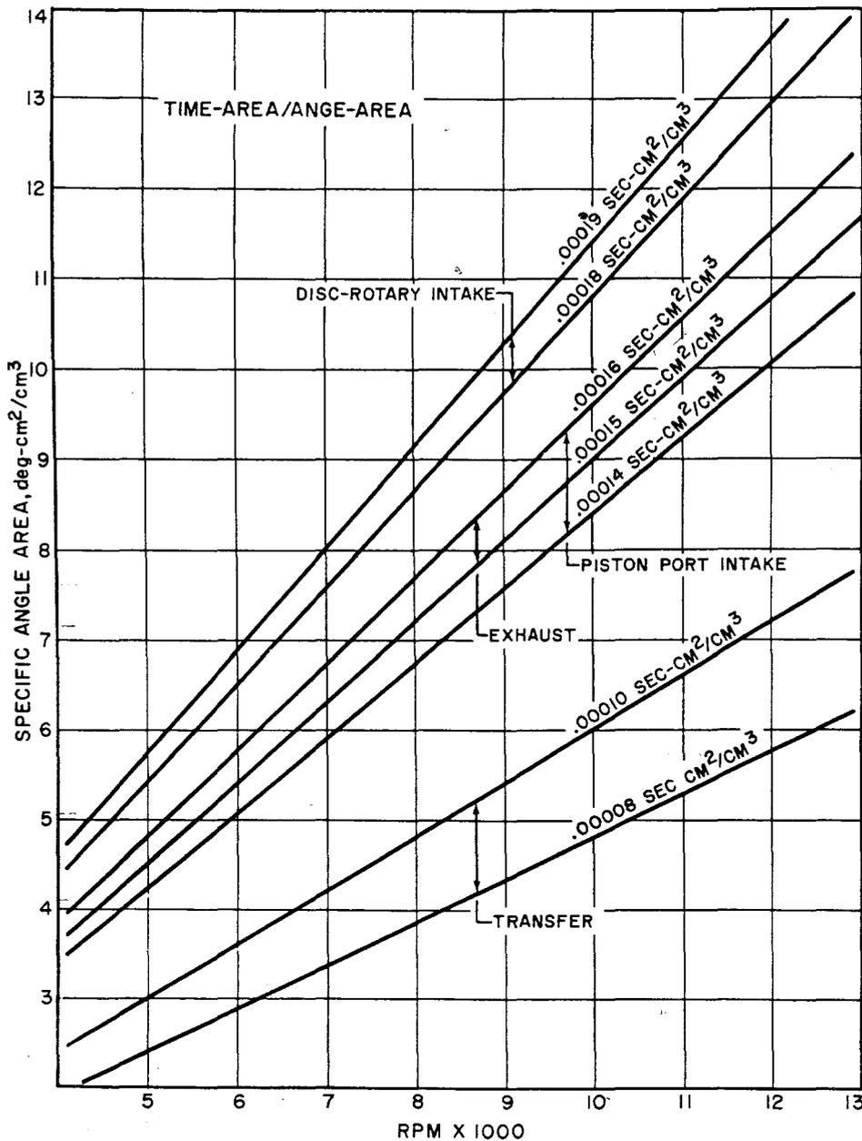
cubic centimeters, (cm<sup>3</sup>), into mean port area, in square centimeters, (cm<sup>2</sup>), and then multiplying the resulting number by the total time, in seconds, (sec), during which the port is open. Combining the formula for calculating time from the port-open period, in degrees, and engine speed, we have:
