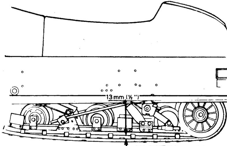
◆ **WARNING: Too much tension will result in power loss and excessive stresses on suspension components.**
