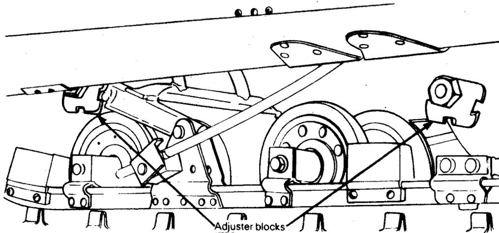
▼ CAUTION: Always turn left side adjuster blocks in a clockwise direction, the right side blocks in a counter-clockwise direction. Left and right adjuster blocks of each adjustment must always be set at the same elevation.
