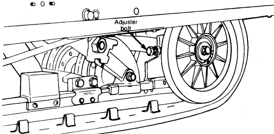
○ **NOTE:** Track tension and alignment are inter-related. Do not adjust one without the other.
