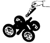
Reassemble entire bogie wheel set, making sure assembly moves freely. Reinstall bogie wheel set. Repeat above steps on remaining bogie wheel sets. Lubricate rear hubs through grease fittings.
