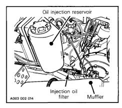
CAUTION: An obstructed injection oil filter will cause oil starvation resulting in serious engine damage.
