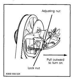
Tighten the lock nut while restraining the other one. Recheck brake light operation.
