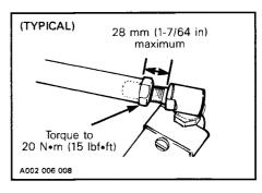
WARNING: The ball joint socket must run parallel with the steering arm. The tie rod must be restrained when tightening the tie rod end lock nuts.
