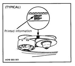
CAUTION: Do not force or use tools to pry the belt into place, as this could cut or break the cords in the belt.
