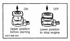
WARNING: For safety reasons, the emergency cut-off switch is easily accessible; be careful not to operate it inadvertently.
