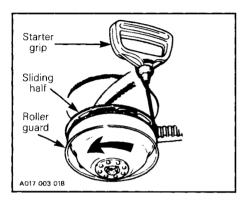
WARNING: Do not wind starting rope around your hand. Hold rope by the handle only.
