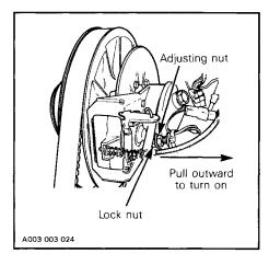
Tighten the lock nut while restraining the other one. Recheck brake light operation.
