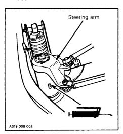
Unhook ski leg boot spring and raise boot to gain access.  Lubricate ski pivot and ski leg lower bushing.
