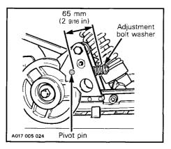
NOTE: The driver can customize this adjustment to meet its particular need. For instance should one is most of the time pulling a load and use rarely the reverse, the rear pivot could be "locked" by fully tighten the adjustment bolt thus getting a better traction and a more positive steering.
