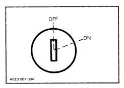
Key operated, two position switch. To start the engine, first turn the key to ON position. To stop the engine, turn the key to OFF position.
