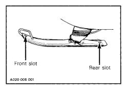
To check, measure the distance between front slots and compare with the distance between rear slots. The front distance should be 3 mm (1/8 in) greather than the rear one when the handlebar is horizontal.
