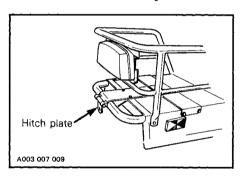
Some vehicles are equipped with a hitch, plate type, on the rear bumper. A hook type may be fitted to the actual hitch. Consult your authorized dealer for details.
