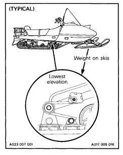
At the highest position, the weight is transferred to the track thus giving a better traction. CAUTION: Always turn the left side adjuster block in a clockwise direction, the right side block in a counterclockwise direction. Left and right adjuster blocks must always be set at the same elevation.
