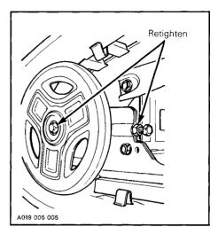
Restart engine, rotate track **slowly** and recheck alignment.
