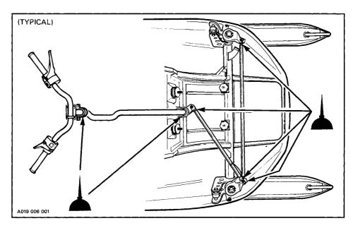
The following lubrication points have to be performed on LH & RH sides:
