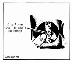
To adjust, loosen lock nut and fully tighten adjuster screw by hand then back off to obtain 4 - 7 mm (5/32 - 9/32'') deflection. Tighten lock nut and recheck chain tension.
