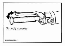
After the adjustment, brake should apply fully when lever is approximatively 13 mm (1/2") from handlebar grip. If not, do not tamper with the brake, contact the dealer.
