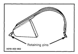
3. Lift and remove the belt guard assembly.
