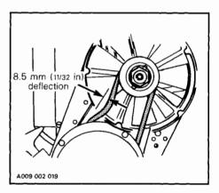
If belt seems damaged or if tension is incorrect, contact an authorized dealer immediately.
