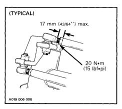
WARNING: The ball joint socket must run parallel with the steering arm. The socket must be restrained when tightening the tie rod end lock nuts.
