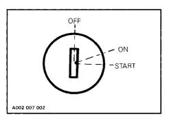
Key, operated, three position switch. To start engine, turn key to START position and hold. Release key to ON position immediately when engine has started. If engine does not start on first try, key must be turned fully back to OFF each time. To stop engine, turn key to OFF position.
