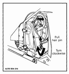
WARNING: If the specified freeplay is not reached with the tensioner screw fully tightened, consult an authorized dealer.
