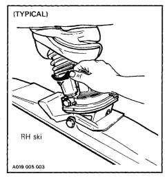
Reinstall boot and secure the spring.
