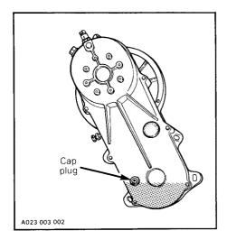
To fill, remove filler plug from top of transmission. Refill as required using Bombardier chaincase oil (P/N 413 8019 00 - 250 ml).
