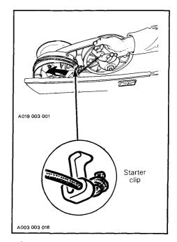
WARNING: Do not wind starting rope around your hand. Hold rope by the handle only.
