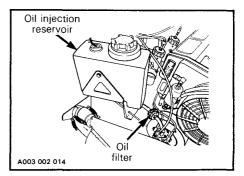
CAUTION: An obstructed injection oil filter will cause oil starvation resulting in serious engine damage.
