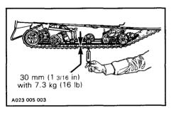
CAUTION: Too much tension will result in power loss and excessive stresses on suspension components.
