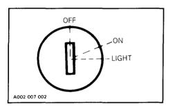
Key operated 3 position switch. To start engine, first turn key to ON position. To stop engine, turn key to OFF position.
