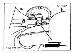
CAUTION: When lubricating the drive axle bearing, do not apply excessive grease as the seal will be pushed out of its housing. Check seal position with finger.
