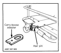
WARNING: When towing a sled or trailer, always ensure to lock the hook with the hair pin.
