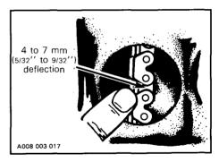
To adjust, loosen lock nut and fully tighten adjuster screw **by hand** then back off to obtain 4 - 7 mm (5/32 - 9/32'') deflection. Tighten lock nut and recheck chain tension.
