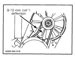
If belt seems damaged or if tension is incorrect, contact an authorized dealer immediately.
