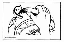
Slip the belt out from the drive pulley and remove completely from vehicle.
