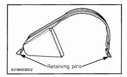
Lift and remove the belt guard assembly.
