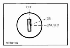
Key operated, 3 position switch. To start the engine, first turn the key to ON position. To stop the engine, turn the key to OFF position.
