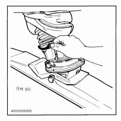
Reinstall boot and secure the spring.
