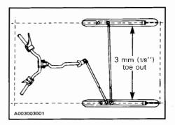
The handlebar should also be horizontal when the skis are pointed toward the front.
