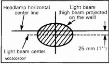
To adjust, remove the four caps, turn upper or lower adjusting screws to obtain desired beam position.
