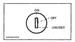
Key operated, 3 position switch. To start engine, first turn key to ON position. To stop engine, turn key to OFF position. The  $3^{rd}$  position is unused.
