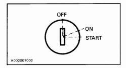
Key operated, 3 position switch. To start engine, turn key to START position and hold. Return key to ON position immediately when engine has started. To stop engine, turn key to OFF position.
