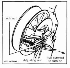
Tighten the lock nut while restraining the other one. Recheck brake light operation.
