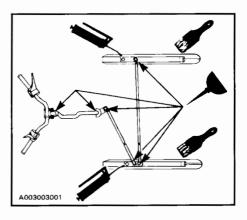
Oil spring coupler bolts, ball joints and steering column bushings.
