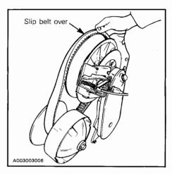
Slip the belt out from the drive pulley and remove completely from vehicle.
