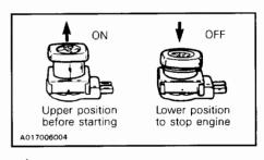
WARNING: For safety reasons, the emergency cut-off switch is easily accessible; be careful not to operate it inadvertently.
