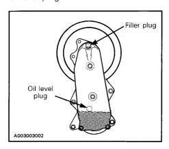
The oil should be level with the bottom of the oil level orifice. Refill as required using Bombardier chaincase oil (P/N 413 8019 00 - 250 ml).
