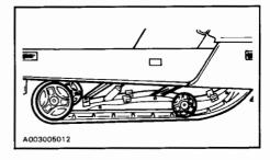
This suspension type does not require any lubrication.
