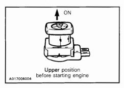
Ensure the tether cut-out cap is in position and that the cord is attached to your clothing.
