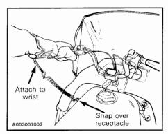
If emergency engine "shut off" is required, completely pull cap from safety switch and engine power will be automatically shut "off".
