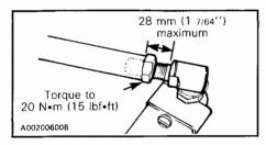
WARNING: The ball joint socket must run parallel with the steering arm. The tie rod must be restrained when tightening the tie rod end lock nuts.
