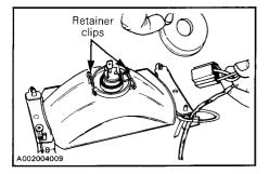
If taillight bulb is burnt, expose the bulb by removing the red plastic lens. To remove, unfasten the two (2) screws.
