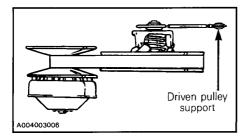
Open the driven pulley by twisting and pushing the sliding half. Hold in fully open position.
