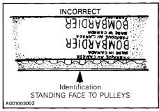
CAUTION: Do not force or use tools to pry the belt into place, as this could cut or break the cords in the belt
