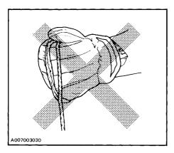
WARNING: Do not start the vehicle by the drive pulley unless it is a true emergency situation. Have the vehicle repaired as soon as possible.
