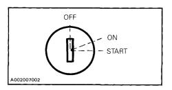
Key, operated, 3 position switch. To start engine, turn key fully clockwise to START position and hold. Return key to ON position immediately when engine has started. To stop engine, turn key counterclockwise to OFF position.
