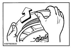
4. Slip slackened belt over the top edge of the sliding half.
