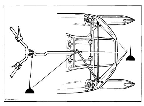
The following lubrication points have to be performed on LH & RH sides:
