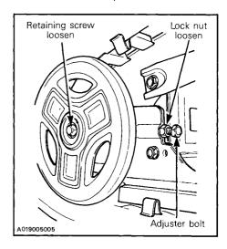
NOTE: Track tension and alignment are inter-related. Do not adjust one without the other.
