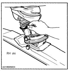
Reinstall boot and secure the spring.
