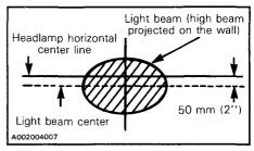
To adjust, remove the four caps, turn upper or lower adjusting screws to obtain desired beam position.
