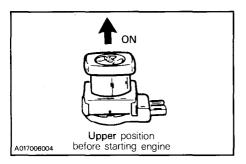
Ensure the tether cut-out cap is in position and that the cord is attached to the clothing.
