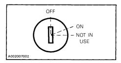
Key operated, 3 position switch. To start the engine, first turn the key clockwise to ON position. To stop the engine, turn the key counter-clockwise to OFF position.
