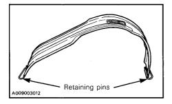
Lift and remove the belt guard assembly.
