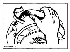
Slip the belt out from the drive pulley and remove completely from vehicle.
