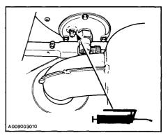
CAUTION: When lubricating the drive axle bearing, do not apply excessive grease as the seal will be pushed out of its housing. Check seal position with finger.
