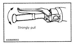
After the adjustment, brake should apply fully when lever is approximatively 13 mm (1/2'') from handlebar grip. If not, do not tamper with the brake, contact an authorized dealer.
