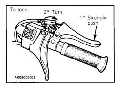
To unlock: Press the lever then turn the device counterclockwise.
