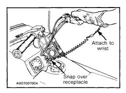
If emergency engine "shut off" is required, completely pull cap from safety switch and engine power will be automatically shut "off".
