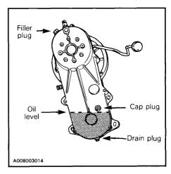
NOTE: Drain plug is accessible through a hole located underneath vehicle.
