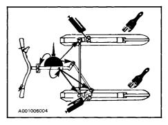
Oil spring coupler bolts, ball joints and steering column bushings.
