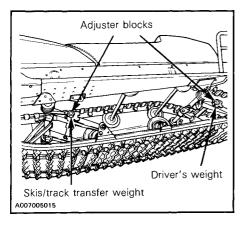
When the front adjuster blocks are at the lowest elevation more weight is distributed on the skis.
