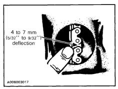
To adjust, loosen lock nut and turn adjuster bolt to obtain the specified free-play. Tighten lock nut and recheck chain tension.
