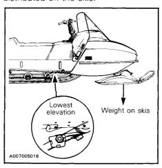
At the highest position the weight is transferred to the track. The rear adjuster blocks should be adjusted to suit the driver's preference.
