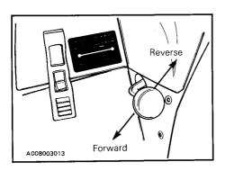
WARNING: This snowmobile is capable of a fast reverse. On first outing, operator should become familiar with this operation by practicing on level ground. Always apply the brake before shifting and come to a complete stop then while holding brake on, change gear. This is particularly important while on a slope. Ensure the path behind is clear of obstacles or bystanders. Fast reverse, while turning, could result in loss of stability.
