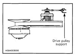
Open the driven pulley by twisting and pushing the sliding half. Hold in fully open position. Slip slackened belt over the top edge of the sliding half.
