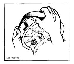
4. Slip the belt out from the drive pulley and remove completely from vehicle.
