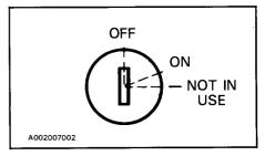
Key operated, 3 position switch. To start engine, turn key fully clockwise to ON position. To stop engine, turn key counterclockwise to OFF position.
