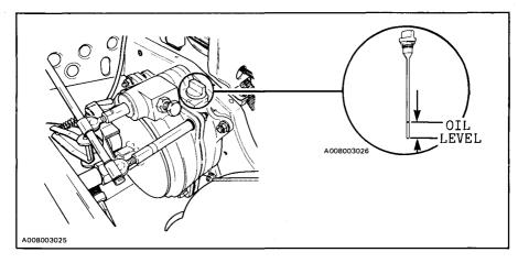
Refill as required using Bombardier chaincase oil (P/N 413 8019 00).
