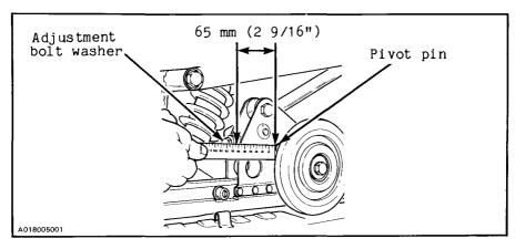
NOTE: If track has an excessive tendency to dig in snow when in reverse, loosen pre-load. Exaggerated loosening of pre-load bolt may cause a loss of traction when moving forward.
