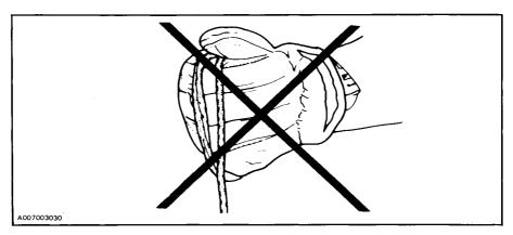
WARNING: Do not start the vehicle by the drive pulley unless it is a true emergency situation. Have the vehicle repaired as soon as possible.
