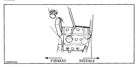
WARNING: This snowmobile is capable of a fast reverse. On first outing, operator should become familiar with this operation by practicing on level ground. Always apply the brake before shifting and come to a complete stop then, while holding brake on, change gear. This is particularly important while on a slope. Ensure the path behind is clear of obstacles or bystanders. Fast reverse, while turning, could result in loss of stability.
