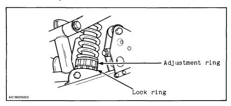
To prevent the rear portion of the track from digging in the snow when in reverse, the slide is hinged and spring loaded at the rear. To check for correct pre-load, measure the distance from the outer edge of the pivot pin to the inner edge of the adjustment bolt washer. The initial adjustment length must be 65 mm (2 9/16").
