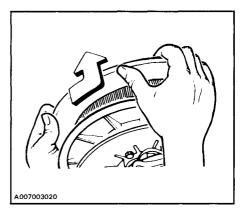
4. Slip slackened belt over the top edge of the sliding half.
