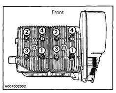
**IMPORTANT:** The engine head nut torque should be checked after the first 5 hours of operation.
