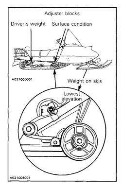
When the front adjuster blocks are at the lowest elevation more weight is distributed on the skis.
