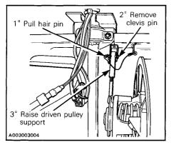
Open the driven pulley by twisting and pushing the sliding half. Hold in fully open position.
