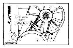
If belt seems damaged or if tension is incorrect, contact the dealer immediately.
