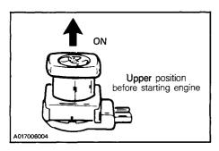
Ensure the tether cut-out cap is in position and that the cord is attached to the clothing.
