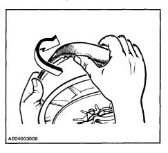
Slip the belt out from the drive pulley and remove completely from vehicle.
