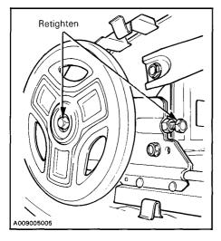
Restart engine, rotate track **slowly** and recheck alignment.
