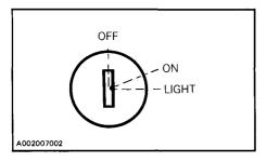
Key operated 3 position switch. To start engine, first turn key clockwise to ON position. To stop engine, turn key counterclockwise to OFF position.
