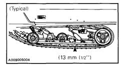
CAUTION: Too much tension will result in power loss and excessive stresses on suspension components.
