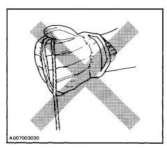
WARNING: When starting the vehicle in an emergency situation by the drive pulley, do not make a knot at the end of the emergency rope and do do not reinstall the belt quard.
