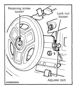
NOTE: Track tension and alignment are inter-related. Do not adjust one without the other.
