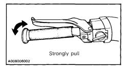
After the adjustment, brake should apply fully when lever is approximatively 13 mm (1/2") from handlebar grip. If not, do not tamper with the brake, contact the dealer.
