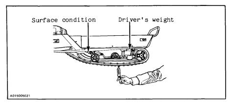
To adjust, use the adjustment key supplied. Spray some WD 40 between spring and spring collar.
