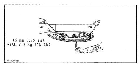
CAUTION: Too much tension will result in power loss and excessive stresses on suspension components.
