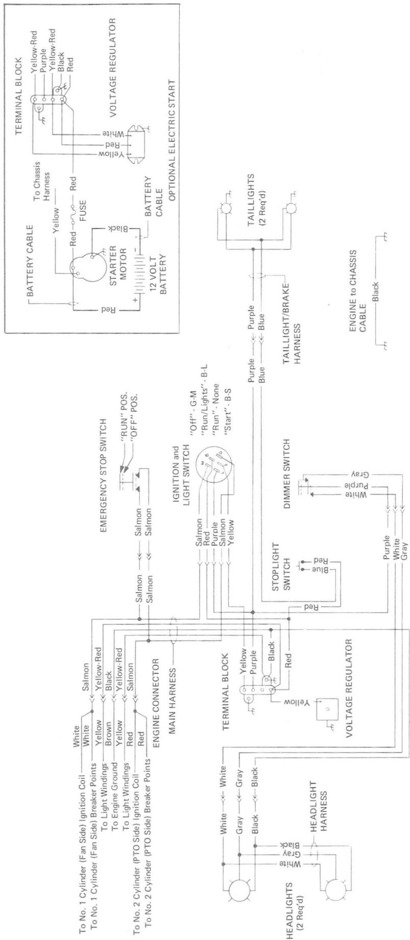
Figure 17. Models 440 M/X and 440 S/R with CHASSIS Serial No. 4064697 and Above Wiring Diagram
