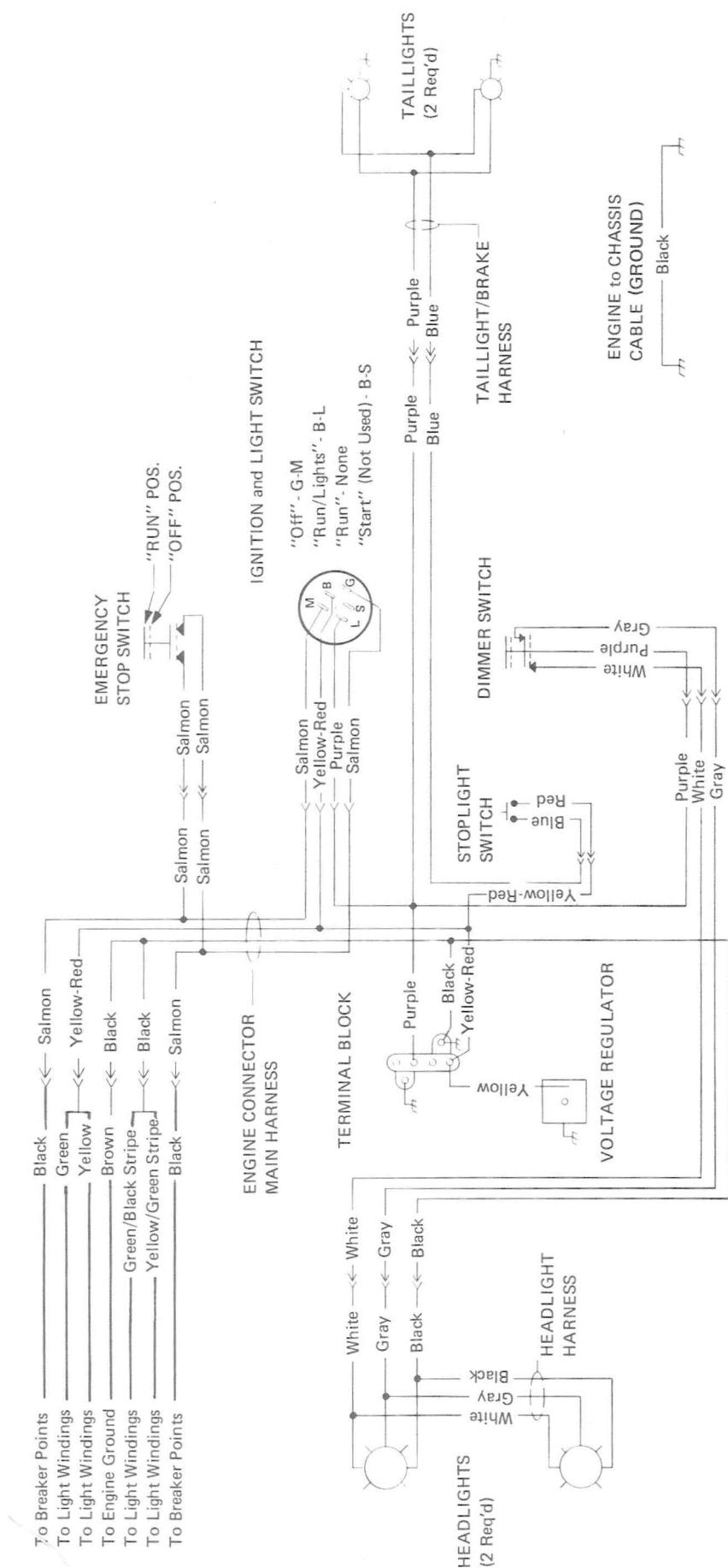
Figure 16. Model 340 S/R Wiring Diagram
