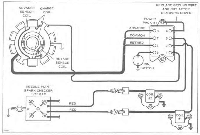
Weak, erratic or no spark from one ignition coil, switch ignition coil leads on Power Pack I - repeat test. Spark on same cylinder still erratic, replace coil. Spark on opposite cylinder erratic, replace Power Pack I.
