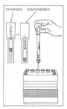
gravity between cells within this range does not indicate a defective battery. Readings should be corrected to 80° Fahrenheit for comparison. If this specific gravity of any cell falls outside this range (1.250 to 1.290), replace the battery.
