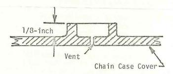
File chain case vent boss on inside of cover down to 1/8-inch height. This will provide necessary clearance for chain tensioner arm.
