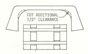
IMPORTANT: File new radius for smooth edge and to prevent cracking.
