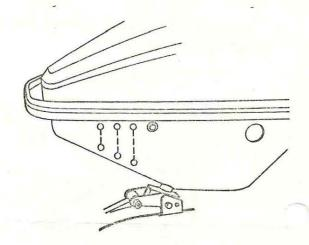
Tape over louver slots if snow tends to build up inside lower pan area.
