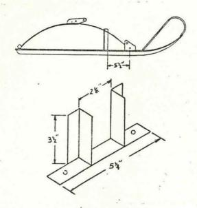
For high speed cornering such as lake races, it is advised to install ski spring stabilizers. Below is a sketch showing the location and needed dimensions to construct your own stabilizers. Use lightweight 1" x 1" angle and 1" flat iron.
