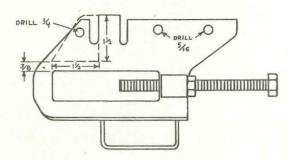
IMPORTANT: Interval weld reinforcing piece to inboard side of rear idler bracket.
