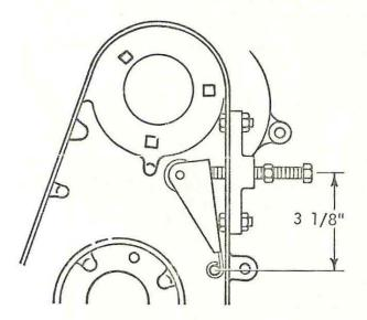
Locate tensioner block mounting to outside surface of chain case by measuring 3-1/8 inches up from lower right-hand cover bolt boss center, to center of tensioner bolt hole. File off parting line flash on outside of chain case in area where block mounts.
