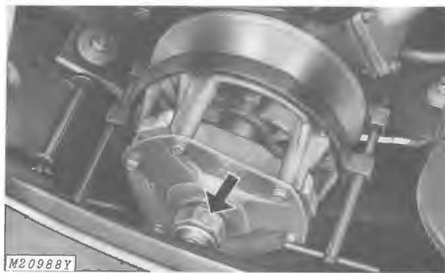
Fig. 4-JDM-41-4 Two-Piece Nut Installed on Hub
