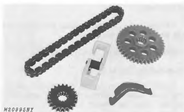
Fig. 12-Drive Chain, Sprockets and Tensioners
