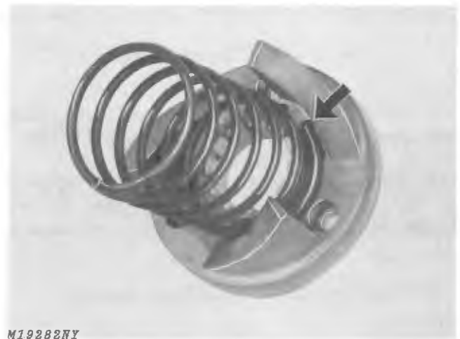
Fig. 15-Spring Installed in Cam
