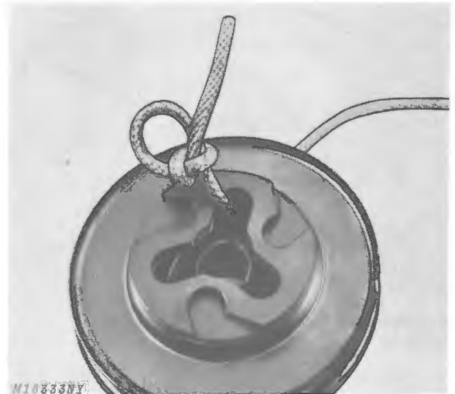
Fig. 9-Installing Rope into Reel
