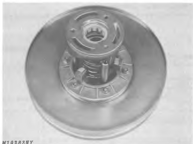
Fig. 16-Installing Cam With Spring on Fixed Face Post
