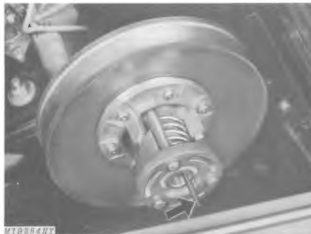
Fig. 17-Installing Driven Sheave on Shaft
