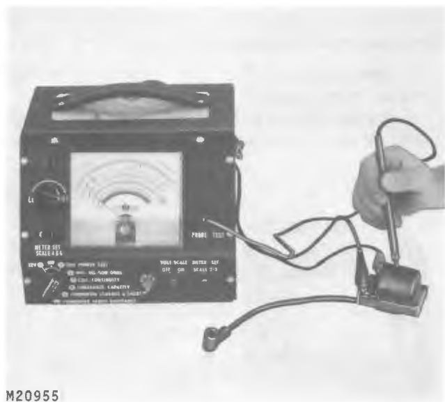
Fig. 13-Testing Ignition Coil Insulation
