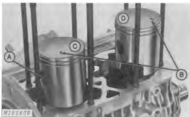
A—Circlip B—Mark C—No. 1 Piston D—No. 2 Piston
