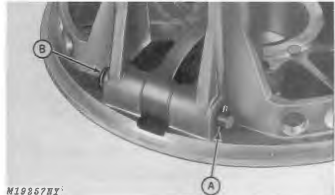
Fig. 10-Removing Spring Pin From Pivot Pin
