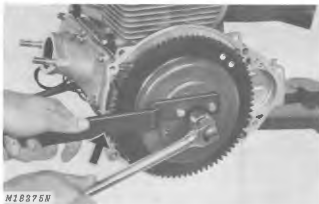
Fig. 16-Removing Flywheel Retaining Nut
