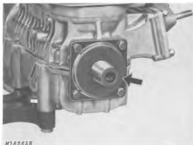
Fig. 29-PTO End Seal Guard
