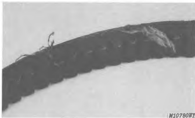
Fig. 4-Drive Belt With Frayed Edge
