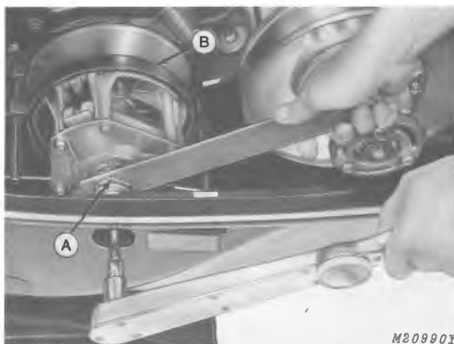
A—JDM-41-4 Two-Piece Nut C—JDM-12-2 Nut Wrench B—JDM-41-2 Compressor Ring
