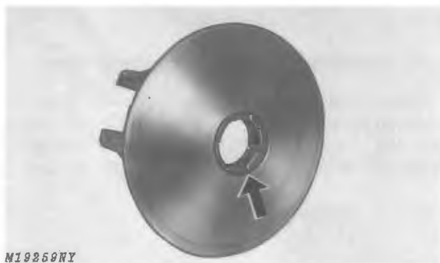
Fig. 12-Cuts in Movable Face Bushing
