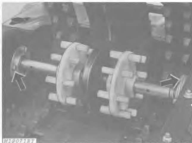
Fig. 22-Installing Drive Shaft - Snowmobile (Serial No. -80,000) Illustrated
