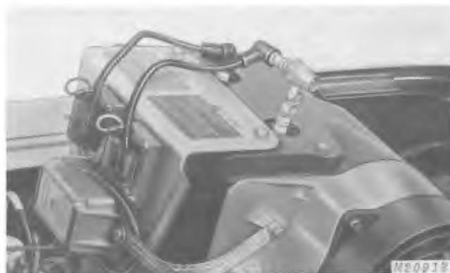
Fig. 10-Testing Ignition Coils With JDM-74A-5 Ignition Tester
