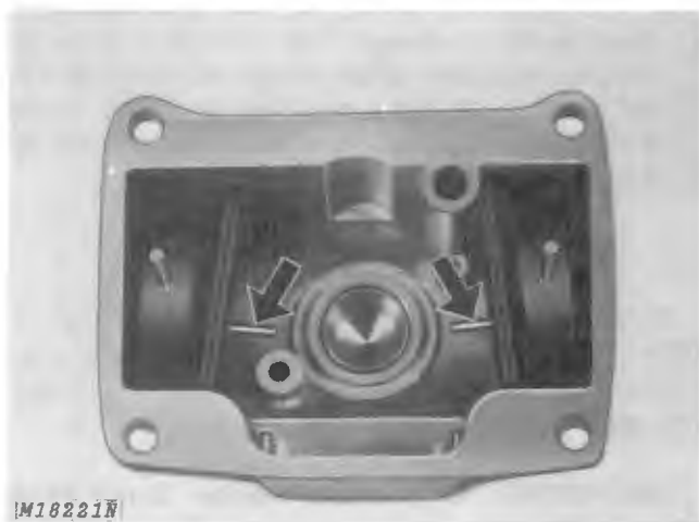
Fig. 16-Positioning Pins When Installing Floats in Float Chamber
