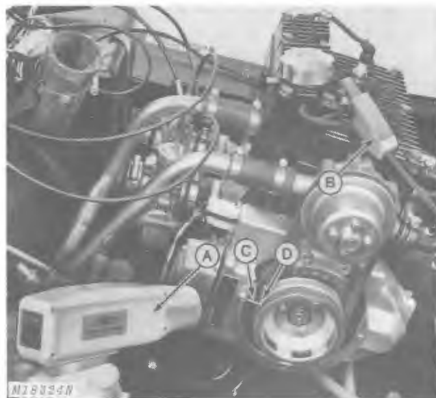
A—Timing Light B—Clamp on Pick-up C—Pointer D—Mark on Flywheel Sheave
