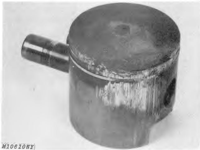
Fig. 6-Melted and Scuffed Piston
