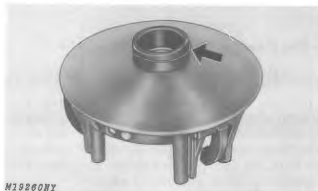
Fig. 13-Snap Ring Position of Movable Face Bushing
