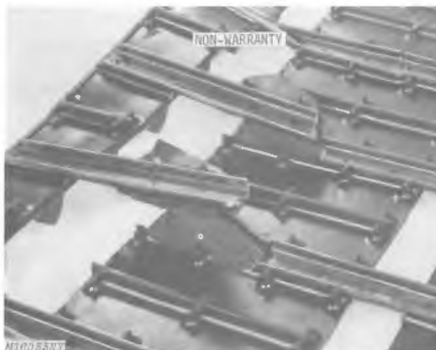
Fig. 7-Grouser Bar Torn from the Track
