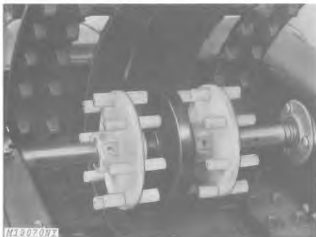
Fig. 19-Drive Wheels Positioned In The Center Snowmobile (Serial No. -80,000) Illustrated
