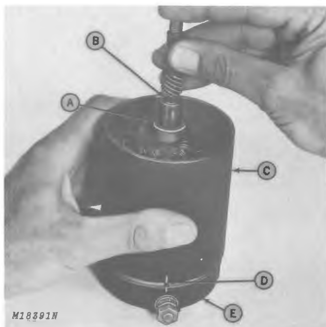
A—Steel Spacer Washer B—Armature C—Housing D—Index Marks E—End Caps
