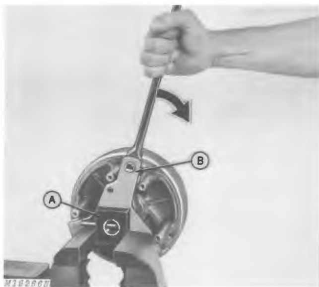
A—JDM-41-5 Hub Lock B—JDM-41-3 Spider Tool
