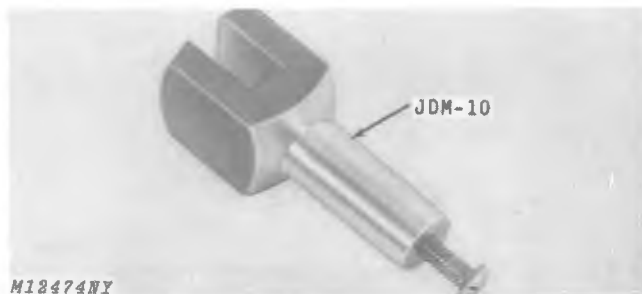
Fig. 6-Dial Indicator Mounting Bracket
