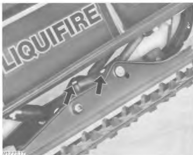
Fig. 17-Steering Response Adjusting Screws
