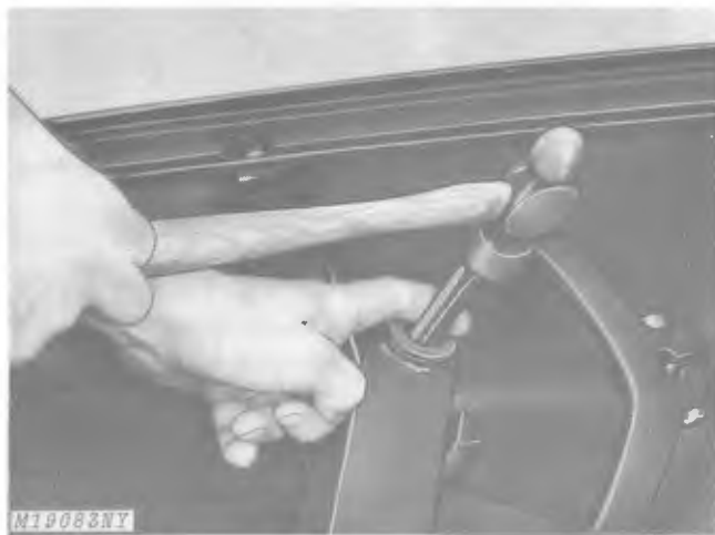
Fig. 11-Removing Steering Spindle Bushings
