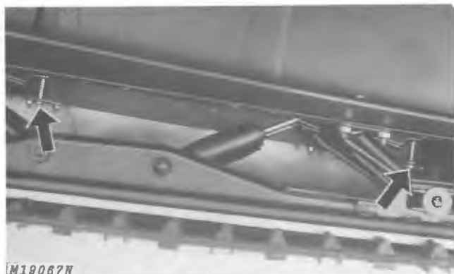
Fig. 16-Suspension Spring Adjusting Screws
