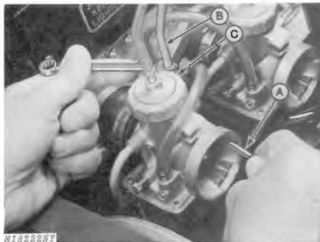
A—JDM-75 Carburetor Choke Gauge C—Jam Nut B—Adjusting Sleeve
