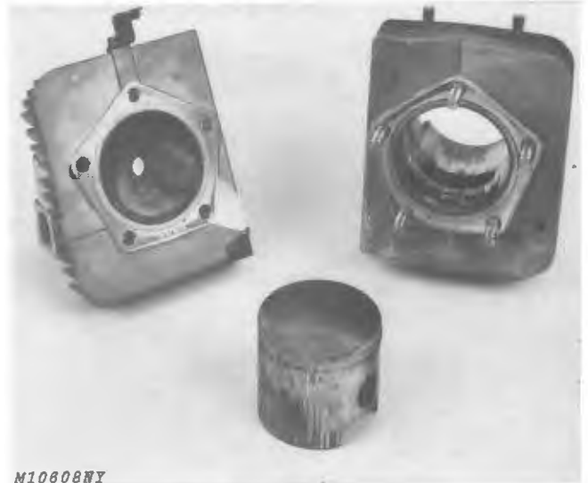
Fig. 4-Piston and Cylinder Scuffing
