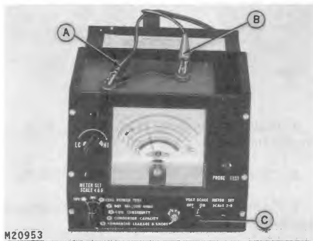
A—Negative Post B—Positive Post C—Volt Scale Switch
