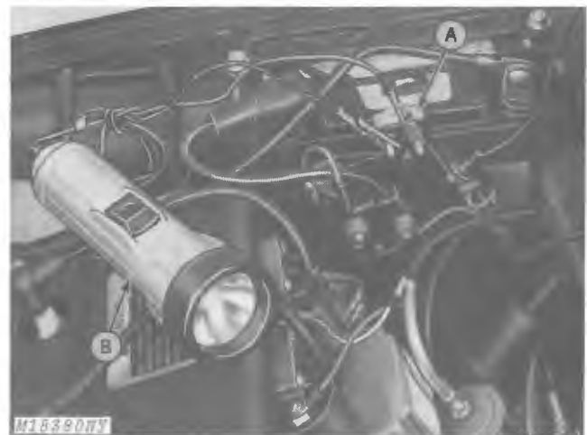
A—Circuit Breaker B—Flashlight Tester
