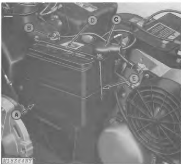
A—Battery Box D—Hold-Down B—Negative Terminal E—Hold-Down Bolt C—Positive Terminal
