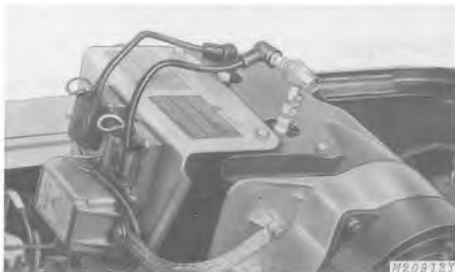
Fig. 1-Checking for Spark at Plug
