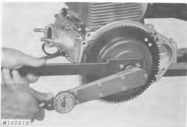
Fig. 19-Installing Flywheel Retaining Nut
