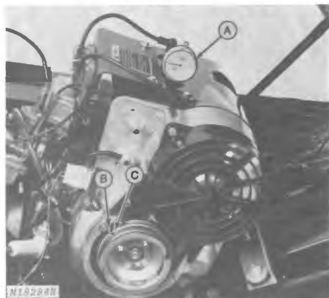
A—Dial Indicator B—Brass Pointer C—Mark on Flywheel Sheave
