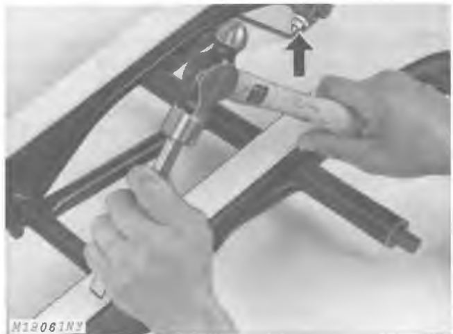
Fig. 8-Removing Slide Rail Wear Bar
