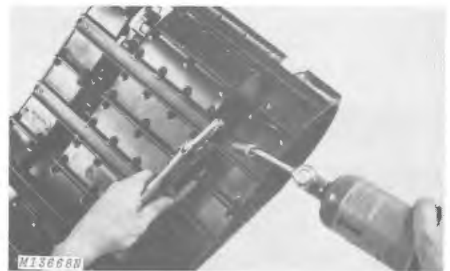
Fig. 15-Removing Grouser Bar (Track Removed for Illustration Purposes)
