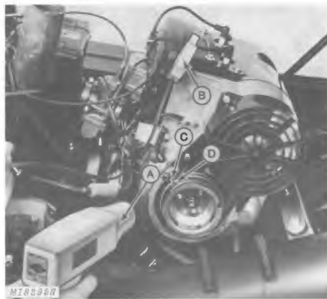
A—Timing Light B—Clamp-on Pick-up C—Pointer D—Mark on Flywheel
