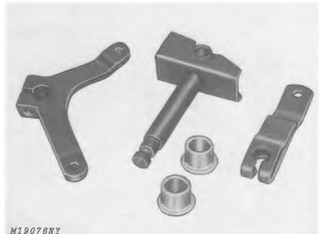
Fig. 4—Steering Arms Spindle and Bushings
