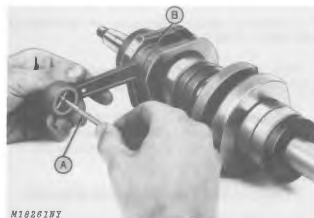
A—Inside Micrometer B—Crankpin Bearing
