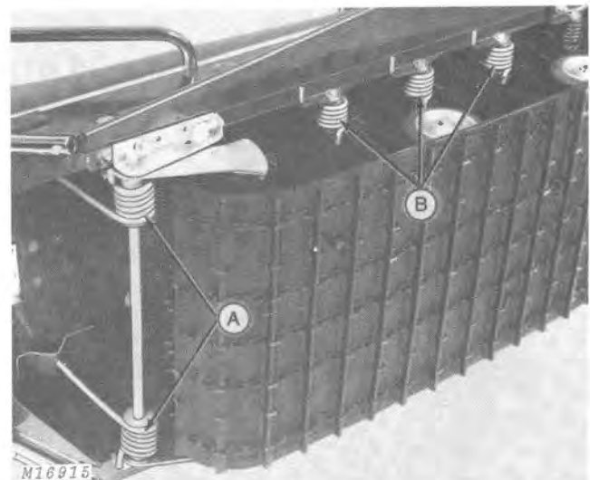
A—Rear Pivot Springs B—Bogie Axle Springs
